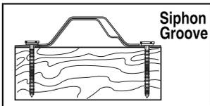
The siphon groove on the underlap of the panel interlocks with the overlap of the next panel, adding strength to the purlin bearing rib. This
